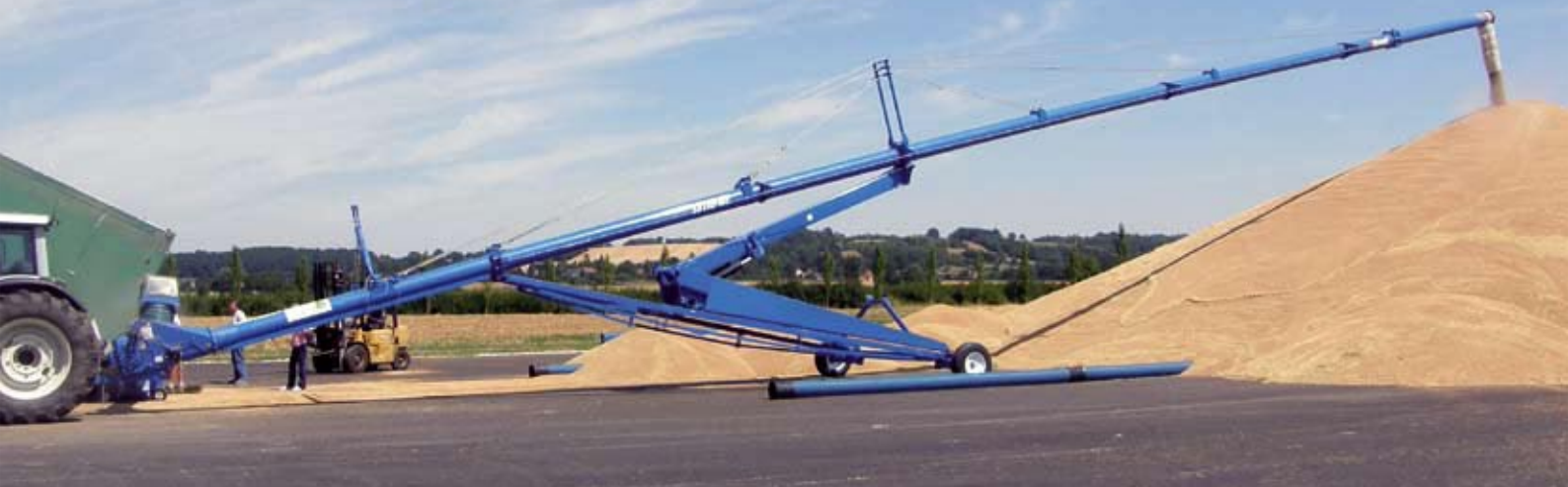
Vis SWING AWAY 13 110HP - Lg = 33.53m 320T/h.
